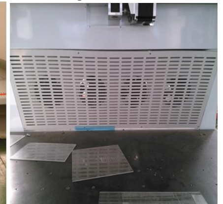
Exhausting Fan for fume outlet
